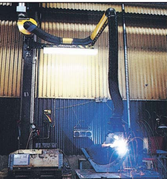
PlymoVent Extractor Crane with an EF-2002/AL-filter, fan and silencer.
