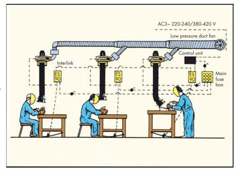
Central System: 3 x LM-2 with individual fans and Energy Savers connected to M-1000 Control Unit and ductwork fan.
